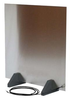
The Vertical Coupling Plate (VCP) is used in conjunction with ESD generators to simulate indirect discharges on metallic objects that are near a test object. The bleeder resistors contained in the ground wire of the VCP serve to prevent the applied charge from vanishing immediately after discharge of the ESD generator to the VCP, thereby increasing the effect of the ESD test.
